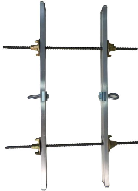
**Description** Rebar Link Bracket for use with the SafeLink Horizontal Lifeline System. Clamps to 12 #9 or larger stirruted rebar, providing two possible anchor points, with 30" rebar rods, 6-1/2 ft above walking/working surface. All associated materials must be rated to meet OSHA, federal, state and local government regulations for fall protection anchor points.
